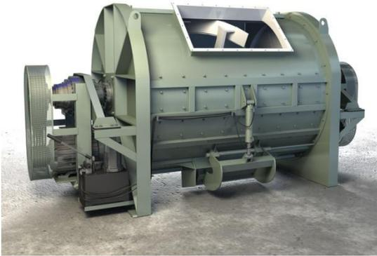
The special mixing action which is realized in the **single shaft system**, thanks to the two opposing ribbons, determines an optimal distribution of the cement paste on each particle of sand and aggregates, the homogeneous distribution of the cement throughout the mix allows a **substantial reduction of the cement required and an increase of the concrete resistance**.
